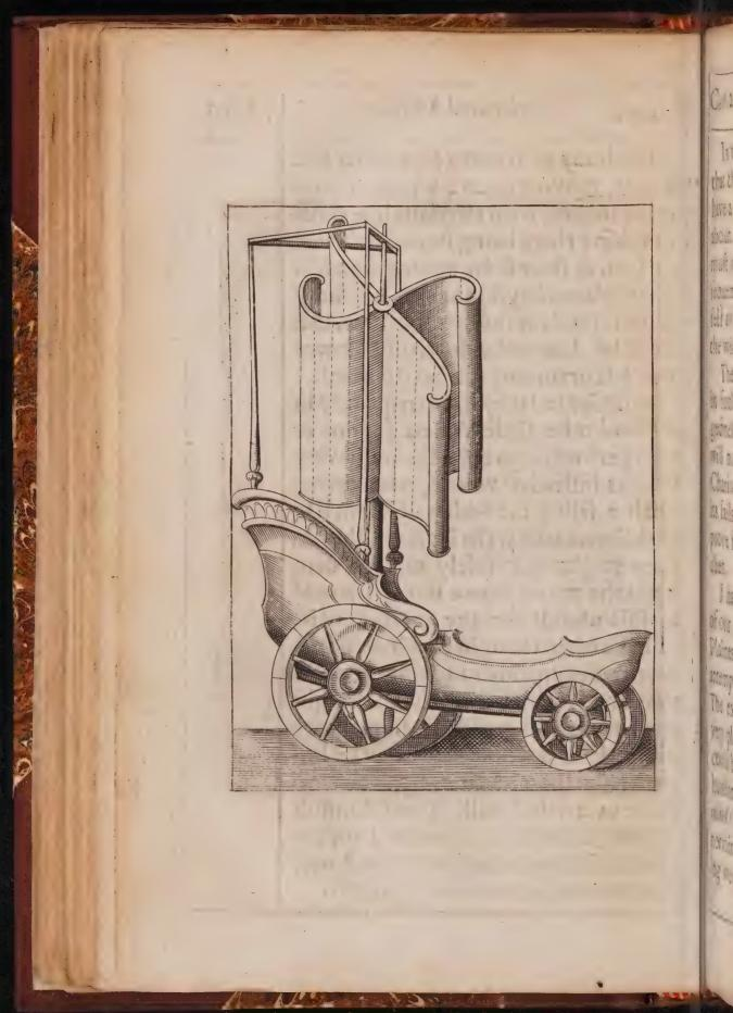
In which the fails are so contrived, that the wind from any Coast will have a force upon them to turn them about, and the motion of these sails must needs turn the wheels, and consequently carry on the Chariot it self to any place (though fully against the wind) whither it shall be directed.
